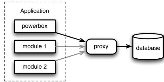
**Figure 1: Diesel’s architecture.** Each module has its own connection object. The powerbox’s connection has no data separation policy; it is a regular connection to the database. The powerbox set restrictive policies on the connections for modules 1 and 2. The proxy multiplexes the connections, so only one connection goes to the database.
